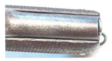
The extractor has been welded and grafted. The WW2 barrel was re-sleeved and grafted and extended in the rear to accept the 7.62 x 25 round. The ejector and the ejection port is slightly modified.
